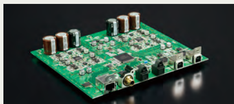
③ D/A converter driving 8 parallel circuits
