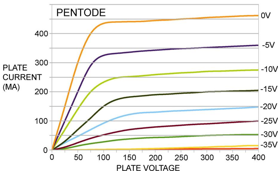
The behavior of an ordinary Jfet or Mosfet is very similar. As with the Pentode, the current flowing from Drain to Source in a Fet will flatten out as the voltage between those pins increases. In this regard Mosfets have a similar shape to the curves of Bipolar transistors, except that Bipolars use input current for control instead of voltage.
