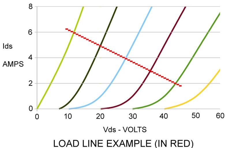
In the original SIT-1 amplifier we put a knob on the front which gave users some control over the load-line setting. It revealed a common preference for what we call a “negative phase 2<sup>nd</sup> harmonic distortion character”. We have settled on this sonic signature as the standard for our SIT amplifiers.
